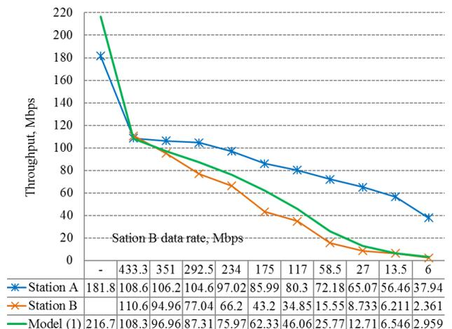
Fig. 5. Stations throughput depending on the data rate of Station B.
