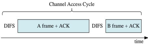
Fig. 1. Time allocation of a channel access cycle.
