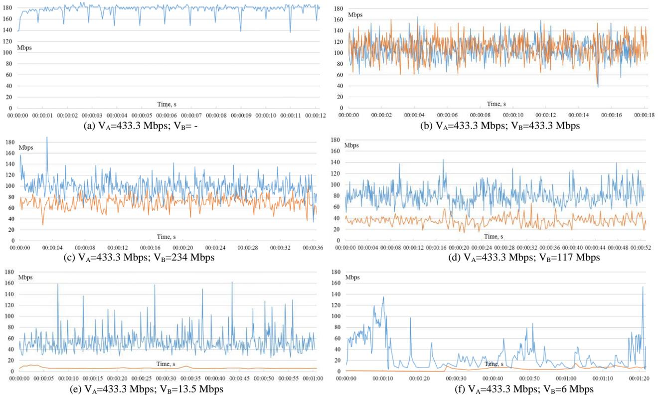
Fig. 6. Results of experimental throughput evaluation depending on stations' data rates: IEEE802.11ac; 80 MHz channel width; MIMO 2x1:1.
