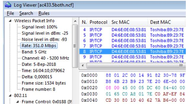
Fig. 4. Packets and physical-layer data captured by *CommView for Wi-Fi*.
