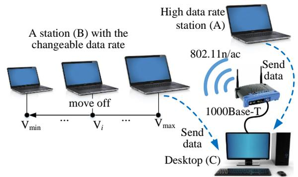
Fig. 2. CSMA/CA airtime distribution between two clients depending on their data rates.
